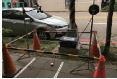
Noise quality monitoring
